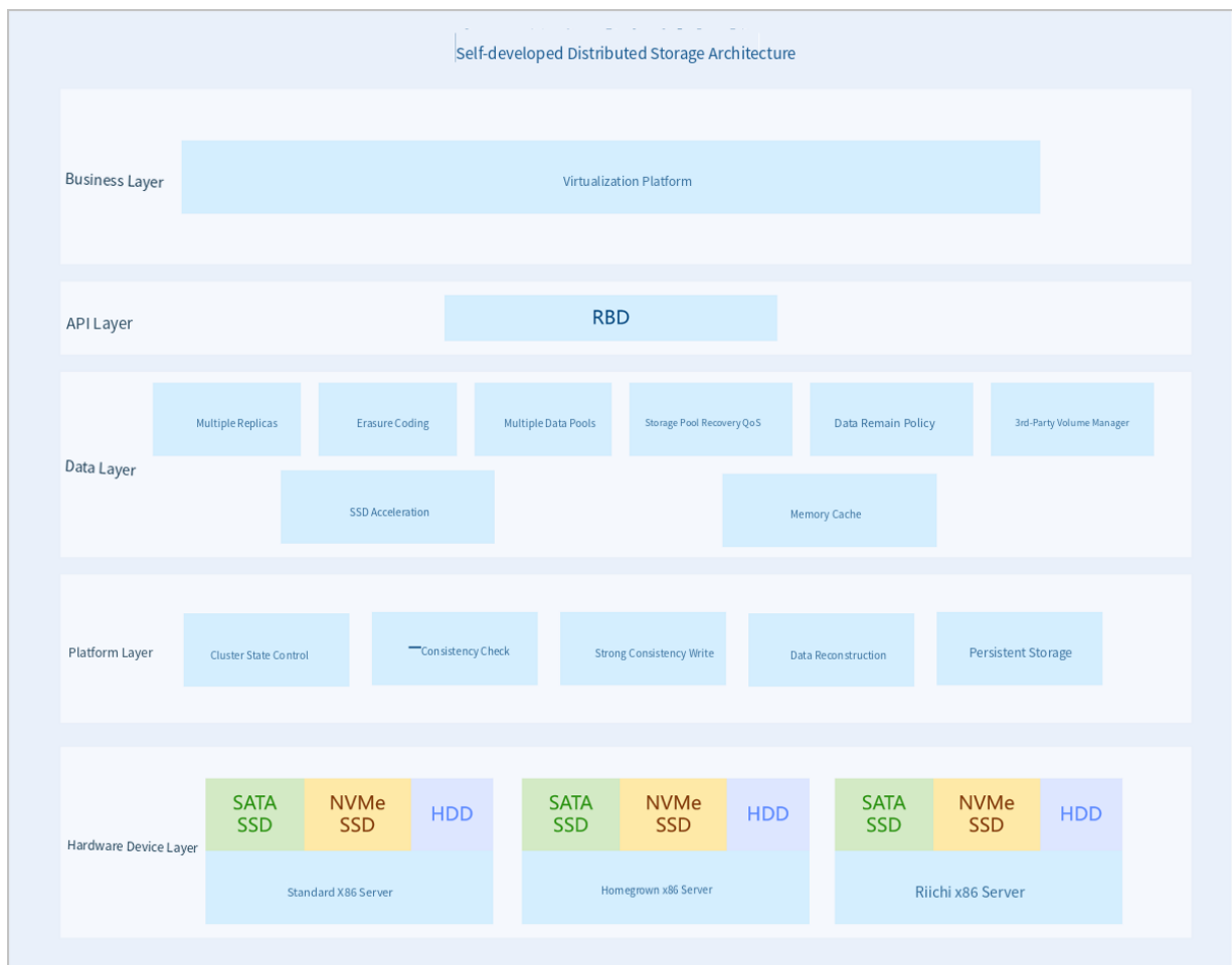
Figure 4-13: Self-developed Distributed Storage Architecture
